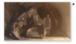
The **intuitive user guidance** supports setting out of the heading direction. Predefined functions, such as positioning of girders, setting out profiles, and configuring the drilling jumbo, **increase productivity**.
