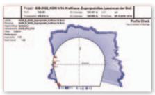
Optimized online graphics allow the tunneling crew to check tunneling progress in real-time. For documentation purposes results are automatically stored as PDF files in the system.
