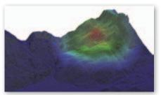
Deformation results are stored as ASCII files and automatically transferred to the office via 2G/3G/4G. The field equipment is permanently monitored. Remote maintenance from the office allows control settings to be adjusted and possible errors to be corrected.
