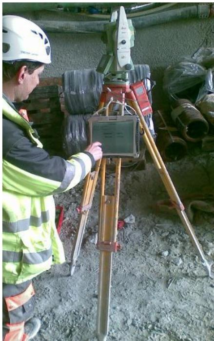
A total of four Axis3D MLS systems are in use in the two tunnels: each tunnel has a permanently installed total station on a console with WiFi and a notebook, as well as a mobile system on a tripod. The notebook and batteries are mounted on the tripod for complete freedom of movement.
