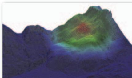
**Deformation results** are stored as ASCII files and **automatically transferred** to the office via 2G/3G/4G. The **field equipment** is permanently **monitored**. Remote maintenance from the office allows control settings to be adjusted and possible errors to be corrected.
