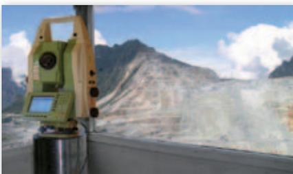
The **stand-alone trigonometric system** continuously measures object coordinates and checks for deformations. Shifts in station coordinates and the influence of refraction are calculated and corrected on-board in the field.
